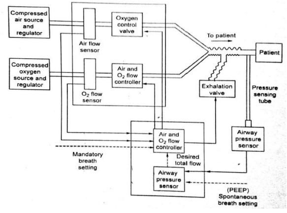
Fig 6.2 Microprocessor based controlled ventilators
