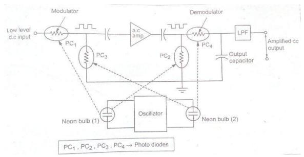
Fig 8.10 Non-mechanical photo conductive chopper amplifier
