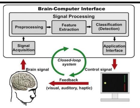
Fig 5.1 Schematic diagram of EEG based BCI
