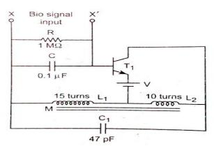
Fig 2.5 Pulsed Hartley oscillator
