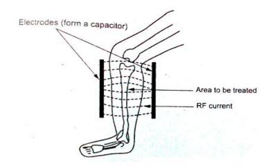
Fig 1.2 Capacitive method
