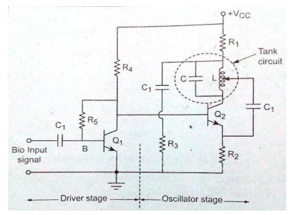
Fig 2.4 Hartley type transmitter
