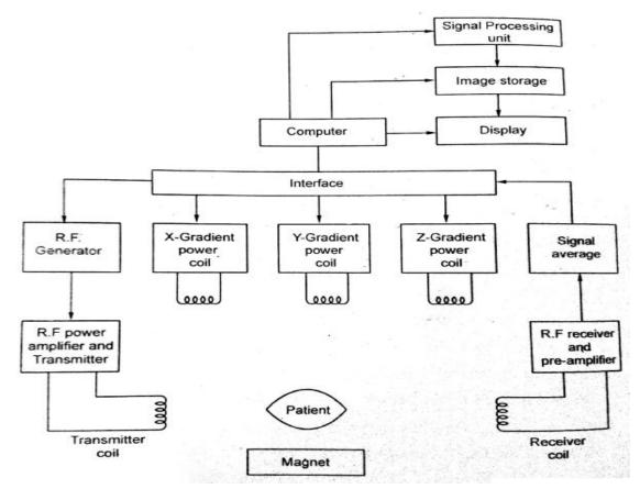
Fig 7.1 Block diagram of MRI system
