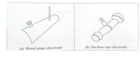
Fig 7.3 – Types of surface electrodes
