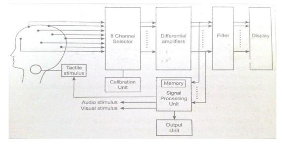
Fig.10.6 Block Diagram of EEG
