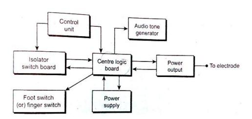
Fig 1.8 Block diagram of electrosurgical diathermy
