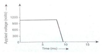
Fig.3.6 Truncated defibrillator discharge waveform
