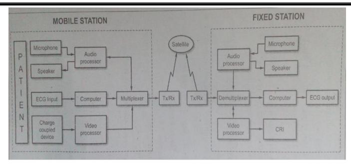
Fig 1.2 Principle of telemedicine using mobile satellite communication
