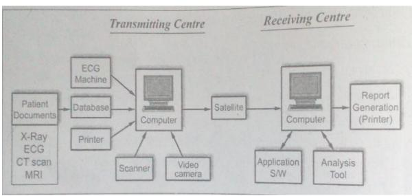
Fig 1.1 Block diagram of a typical telemedicine system
