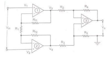
Fig 8.8 Circuit of Instrumentation amplifier
