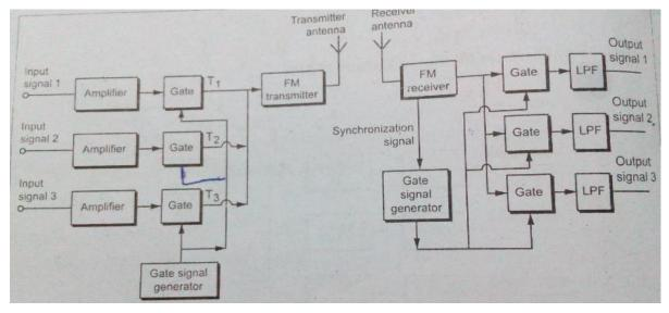
Fig 2.8 Time Division Multiplex Telemetry System
